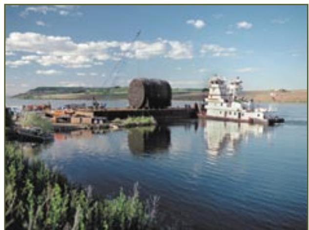
*Defueled reactor components from nuclear-powered submarines and cruisers are barged to the Hanford Site and placed in a trench in the 200-East Area.*
