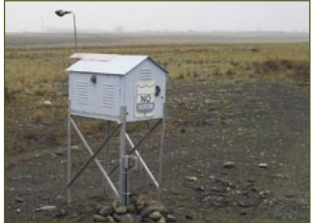
*Air samplers on the site were located primarily around major operational areas to maximize the ability to detect radiological contaminants resulting from site operations.*
