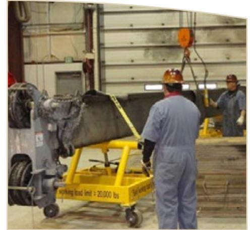
Heavy equipment mechanics disassemble the boom on a 40-ton Grove crane to adhere to the annual inspection requirements.
